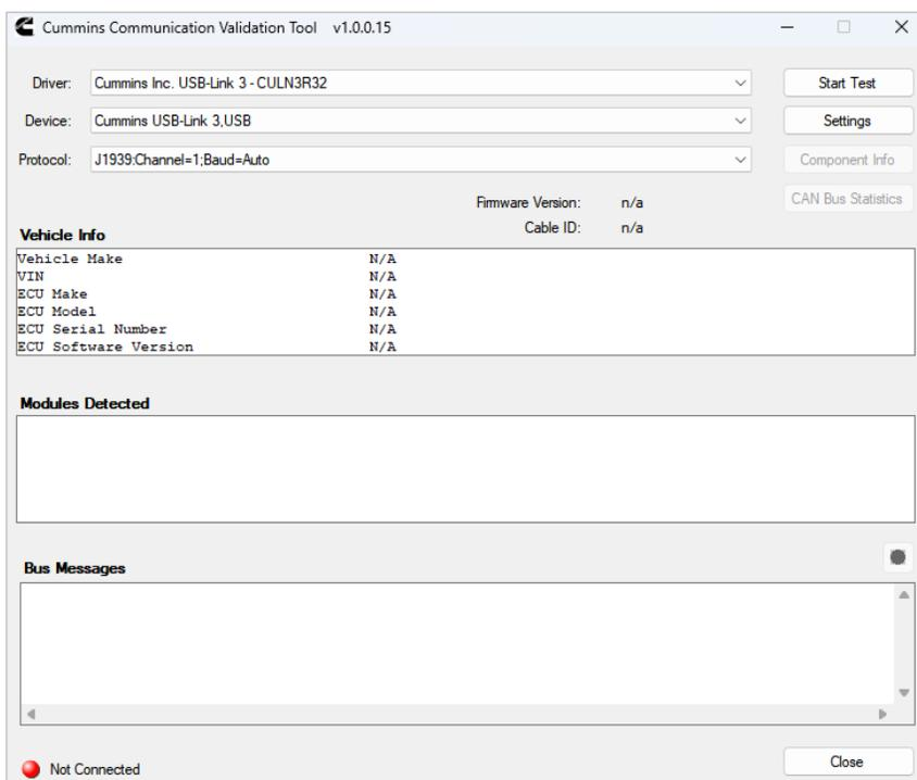
**Figure 3.15** Cummins Validation Tool: Status Not Connected
